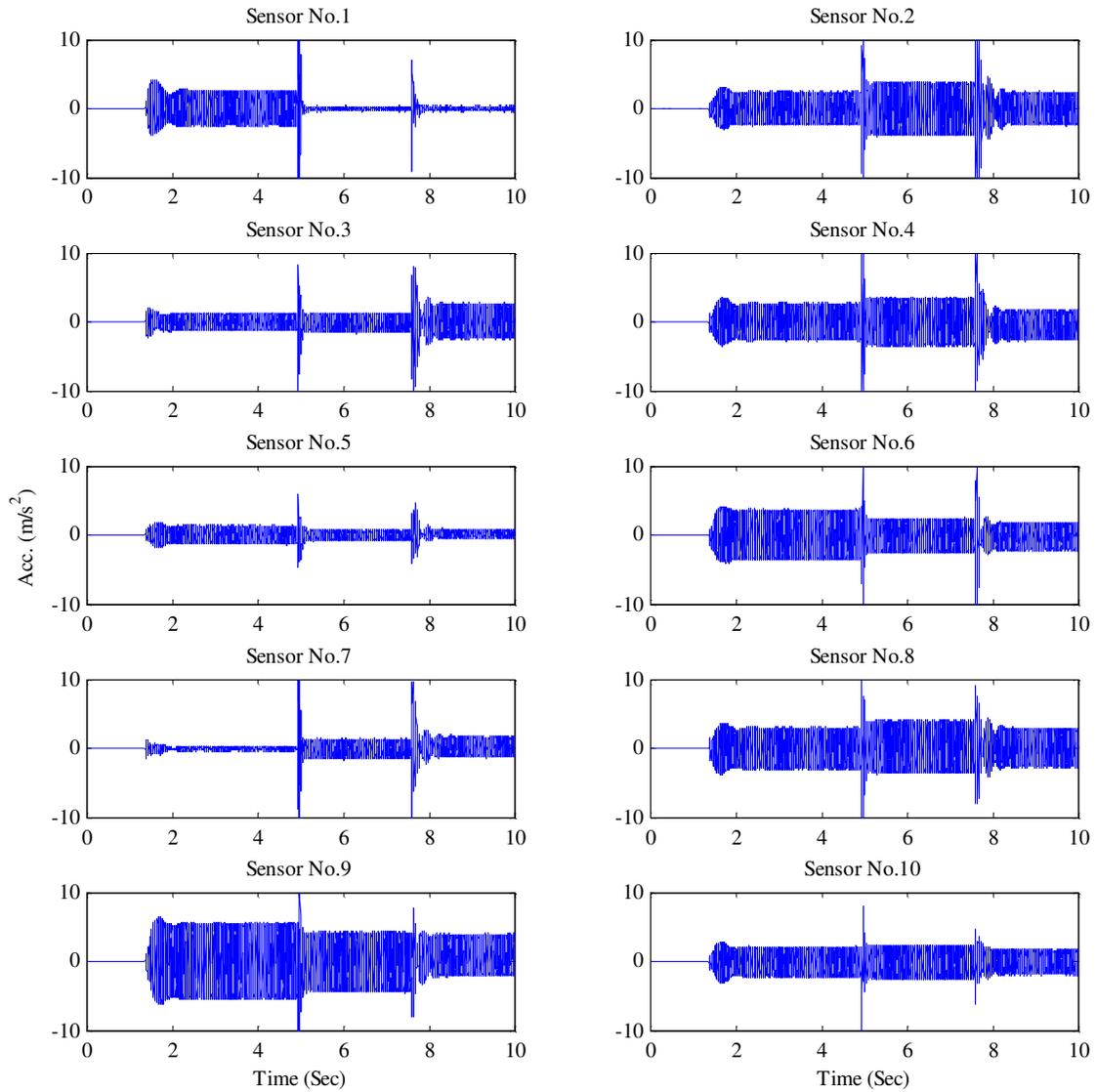
Fig. 4. Response of all 10 sensors on the plate without control, and after controlling with one and then two piezoelectric actuators.
