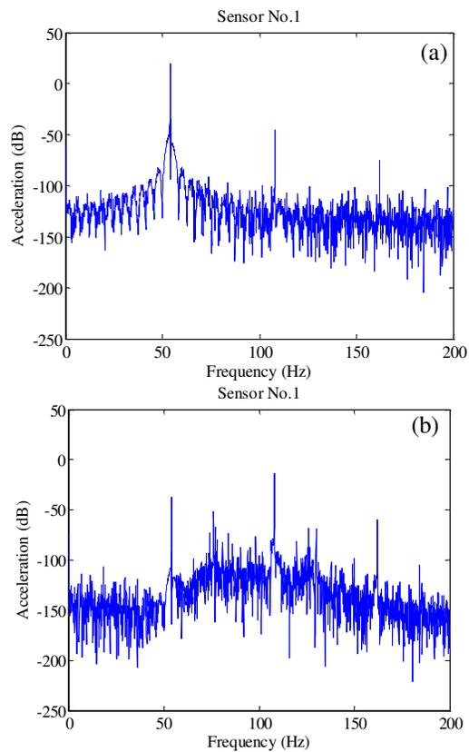
Fig. 5. Frequency response of Sensor No.1 to periodic disturbance with 53 Hz frequency; a) without control, b) controllers for both piezoelectric patches are on.
