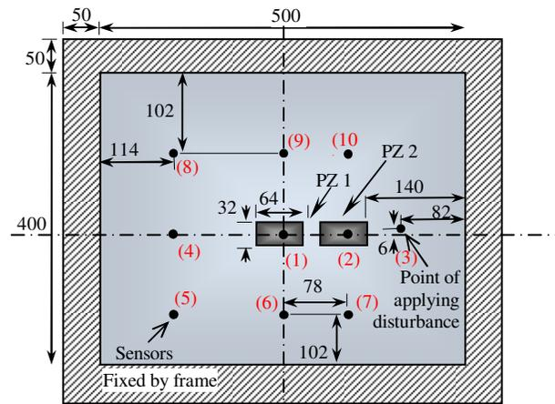
Fig. 1. Schematic of the plate; the unit is millimeter.
