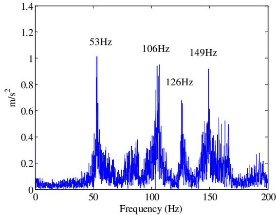
Fig. 3. Frequency response of the plate to a chirp excitation.
