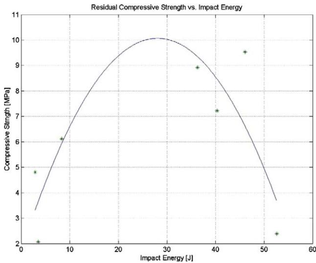
Fig. 14. Residual strength with respect to impact energy (4-ply carbon laminate).
