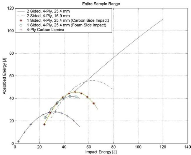
Fig. 4. Impact energy as compared to absorbed energy.
