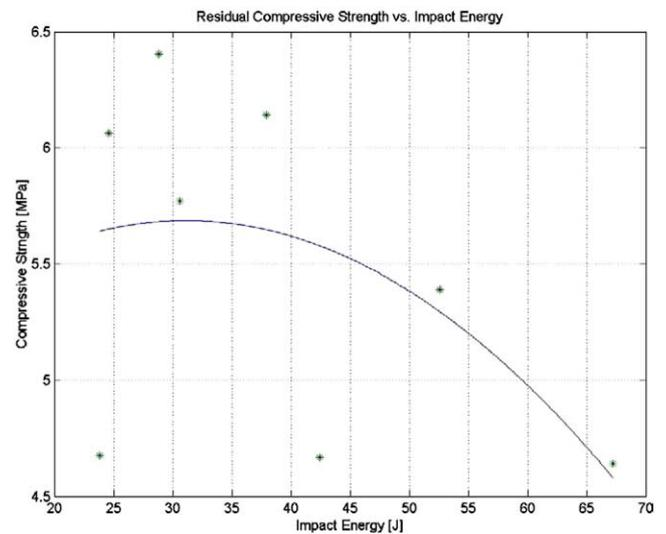
Fig. 12. Residual strength with respect to impact energy (25.4 mm core/l face-sheet, carbon side).
