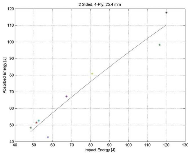
Fig. 7. Impact energy with respect to absorbed energy (25.4 mm core/2 face-sheets).
