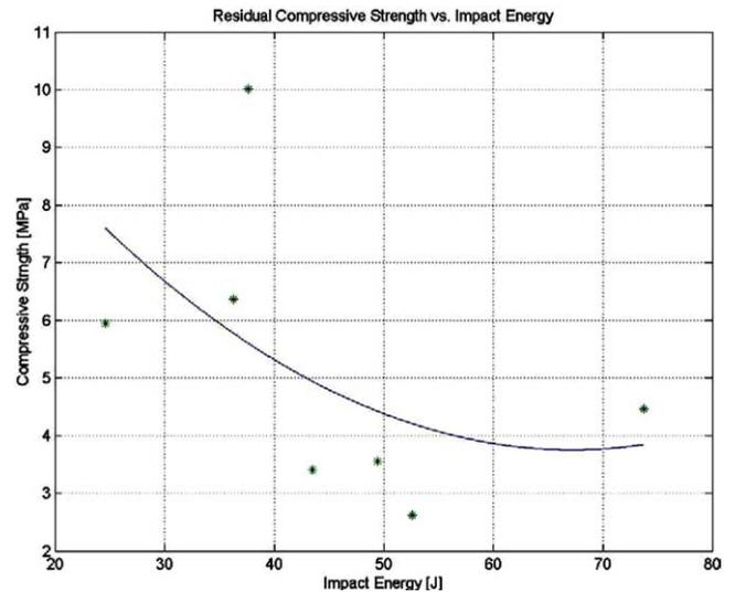
Fig. 11. Residual strength with respect to impact energy (25.4 mm core/l face-sheet, foam side).
