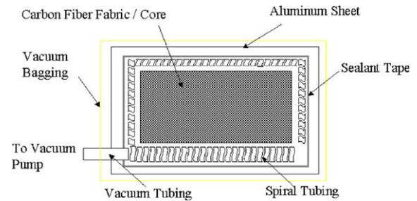
Fig. 1. Manufacturing set-up.
