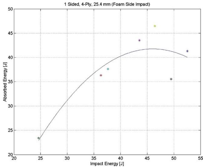
Fig. 10. Impact energy with respect to absorbed energy (25.4 mm core/l face-sheet, foam side).
