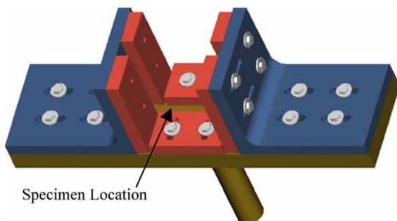
Fig. 3. Compression after impact fixture.
