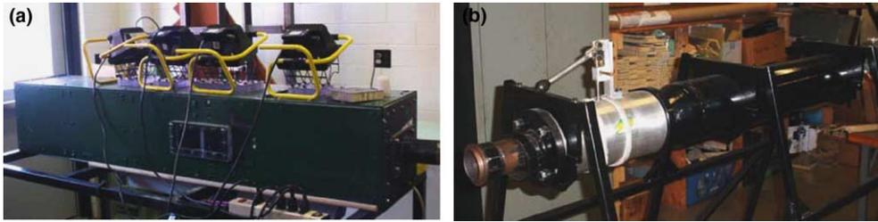
Fig. 2. (a) Pneumatic gun sample chamber. (b) Pneumatic gun firing mechanism.
