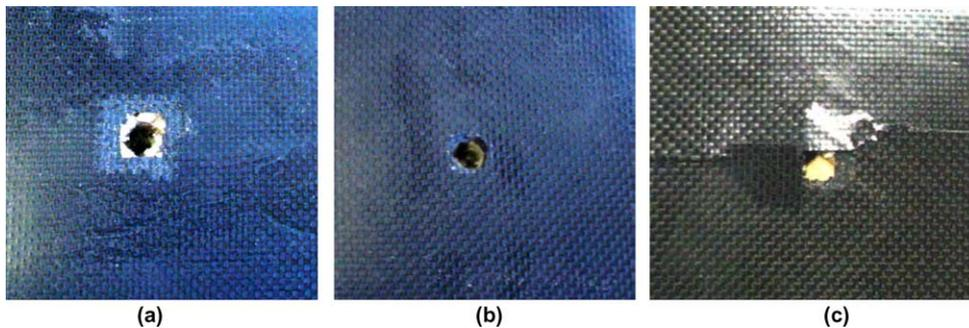
Fig. 15. Non-impacted side damage (25.4 mm core, two face-sheets/120 J impact). Impact side damage (25.4 mm core, two face-sheets/120 J impact). Compression (after impact) damaged sample (15.9 mm core, two face-sheets/43 J impact). (a) Non-impacted side damage (25.4 mm core, two face-sheets/120 J impact). (b) Impact side damage (25.4 mm core, two face-sheets/120 J impact). (c) Compression (after impact) damaged sample (15.9 mm core, two face-sheet/43 J impact).
