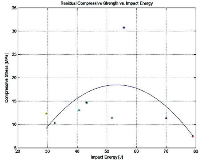
Fig. 6. Residual strength with respect to impact energy (15.9 mm core/2 face-sheets).
