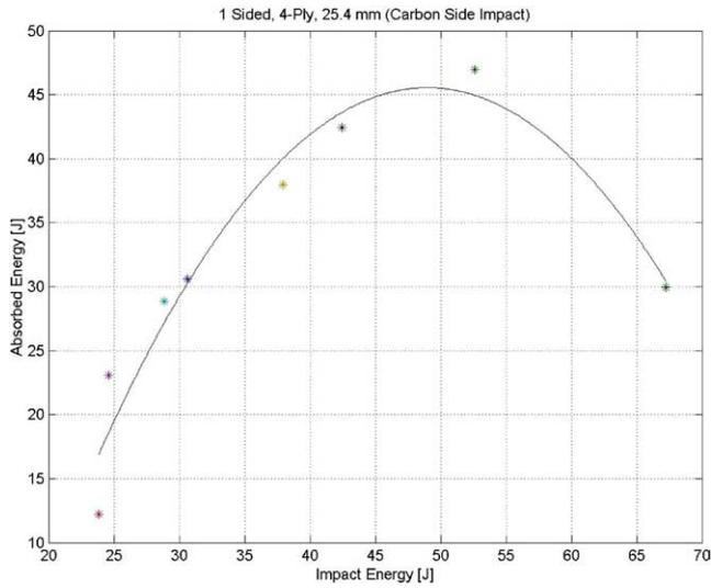
Fig. 9. Impact energy with respect to absorbed energy (25.4 mm core/l face-sheet, carbon side).
