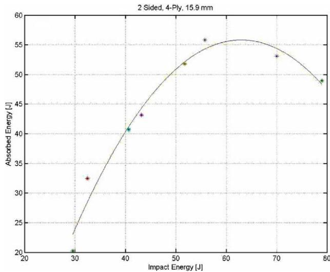
Fig. 5. Impact energy with respect to absorbed energy (15.9 mm core/2 face-sheets).
