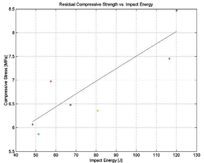
Fig. 8. Residual strength with respect to impact energy (25.4 mm core/2 face-sheets).
