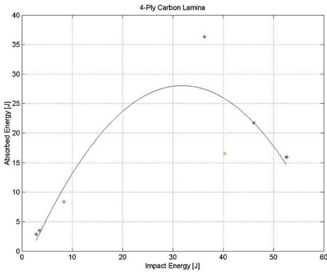
Fig. 13. Impact energy with respect to absorbed energy (4-ply carbon laminate).
