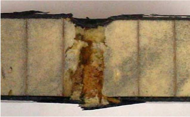
Fig. 16. 25.4 mm sample after 120 J impact and compressive failure.
