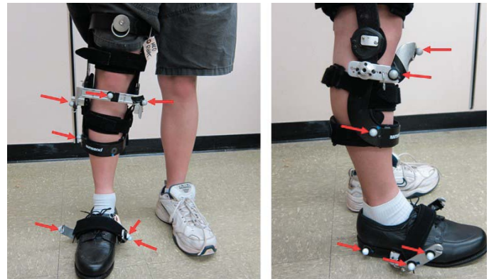
FIGURE 1. KNEE BRACE AND SHOE WITH REFLECTORS. THE ARROWS POINT TO THE VISIBLE REFLECTORS.
