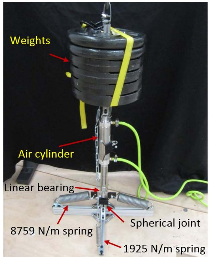
Fig. 3: Mockup and its main components.
