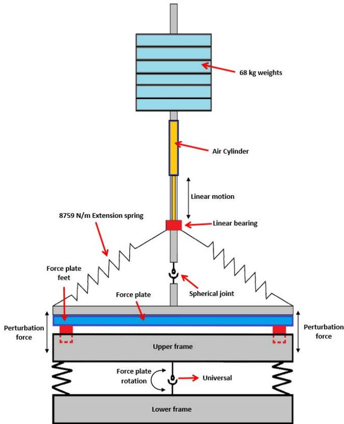
Fig. 2: Side view schematics of the mockup and force plate module. The actuation module generates forces that cause the force plate to rotate and apply perturbation to the mockup in two DOFs.
