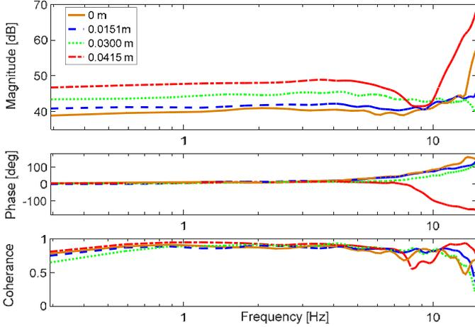
Fig. 6: Impedance of the mockup at different air cylinder positions.
