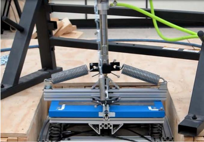
Fig.4: Mockup at its minimum stiffness arrangement.
