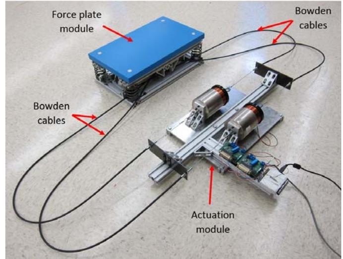
Fig. 1: Vibrating platform and its main modules.
