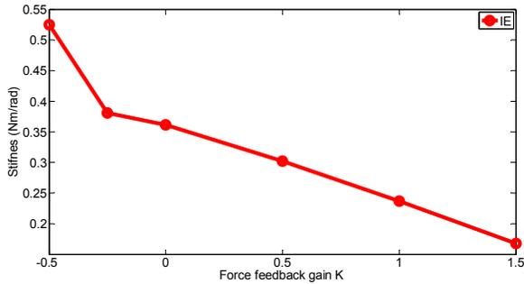
Figure 8. Ankle stiffness in IE at different IE torque feedback gains.
