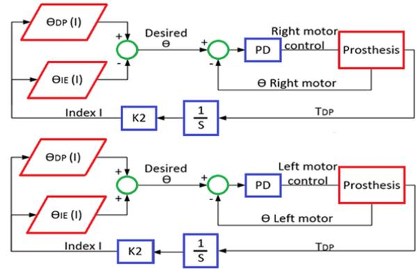
Figure 4. Admittance controllers for the left and right motors. The reference angle for the left motor controller is the sum of the DP and IE angles, while for the right motor controller it is the difference between DP and IE angles. The admittance controller uses the torque feedback in DP ( $T_{DP}$ ) to update the lookup table index  $I$ .
