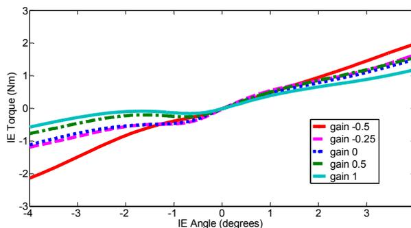
Figure 7. IE torque-angle relationship in the prosthesis with impedance control and different torque feedback gains. Negative angles are plantarflexion, positive angles are dorsiflexion.
