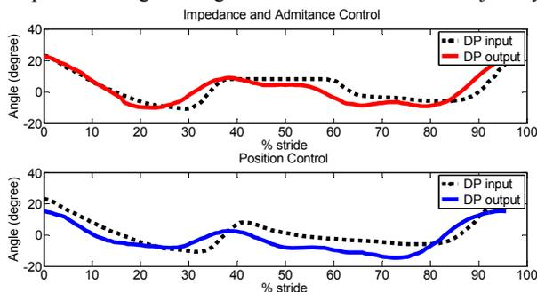
Figure 12. Input and output (compensated for 75 milliseconds time delay) of the ankle trajectory in DP during a representative gait cycle with admittance and impedance control.
