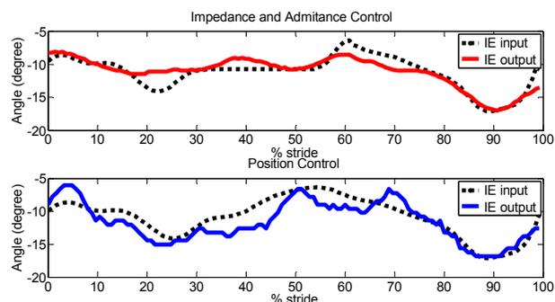
Figure 13. Input and output (compensated for 75 milliseconds time delay) of the ankle trajectory in IE during a representative gait cycle with admittance and impedance control.
