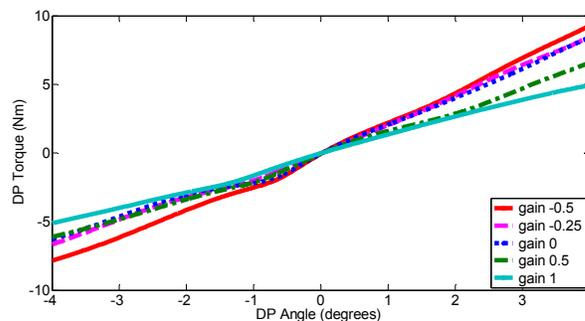
Figure 5. DP torque-angle relationship in the prosthesis with impedance control and different torque feedback gains. Negative angles are plantarflexion, positive angles are dorsiflexion.
