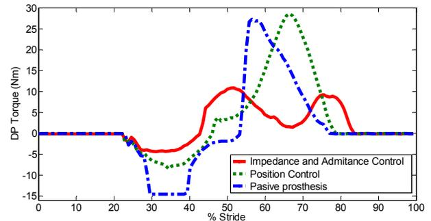
Figure 10. Ankle external torque in DP during a representative gait cycle with different control strategies. Negative torques induce plantarflexion (heel-strike) and positive torques induce dorsiflexion (push-off). With the passive prosthesis, the data acquisition system saturates during heel-strike at -15 Nm torque.
