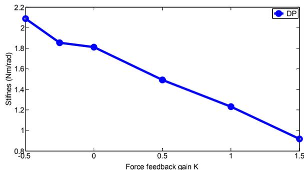
Figure 6. Ankle stiffness in DP at different DP torque feedback gains.
