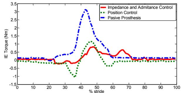
Figure 11. Ankle external torque in IE during a representative gait cycle with different control strategies. Negative torques induce eversion and positive torques induce inversion.
