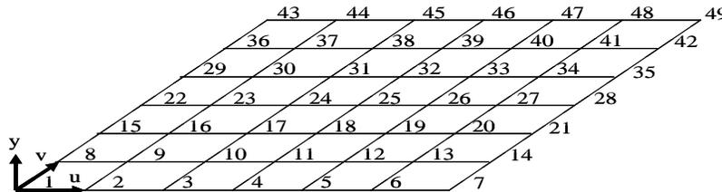
**Figure 3.** Simply supported plate with 49 nodes and 36 elements
