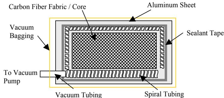
Figure 1. Sample construction setup
