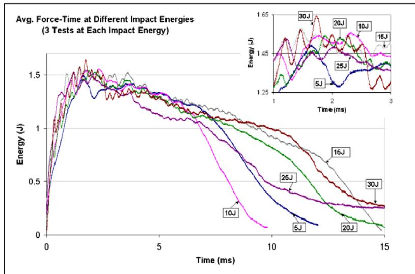
Figure 5. Force vs. Time response for 1-sided, FF, carbon fiber impacted first
