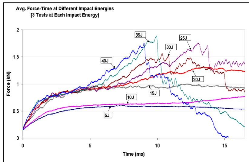
Figure 6. Force vs. Time response 1-sided, FF, foam impacted first
