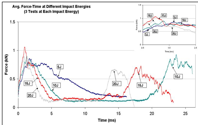
**Figure 9. Force vs. Time response for 2-sided, HH**
