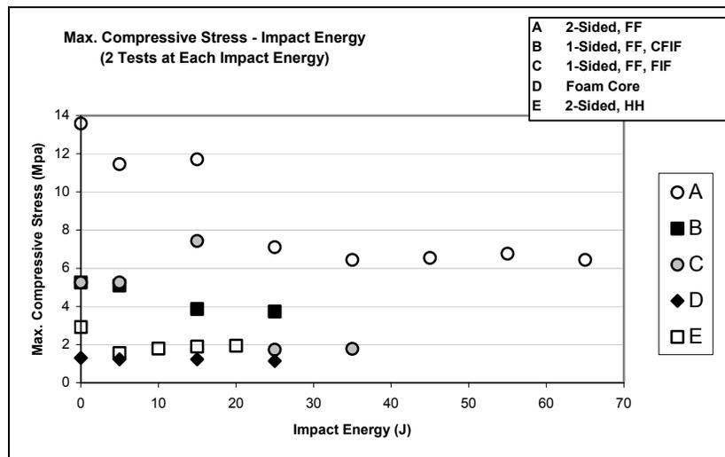
Figure 10. Max. Compressive Stress vs. Impact Energy
