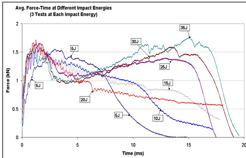
Figure 7. Force vs. Time response 2-sided, FF (Impact Energies 5-35J)
