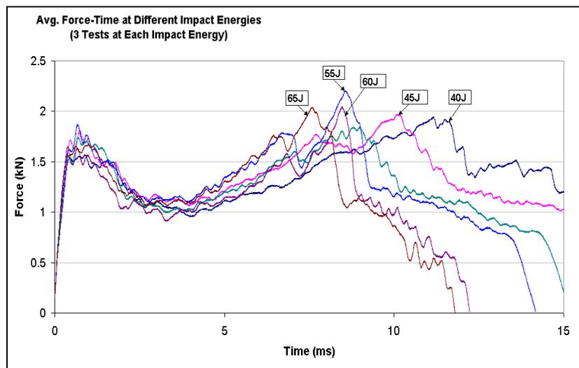
Figure 8. Force vs. Time response 2-sided, FF (Impact Energies 40-65J)
