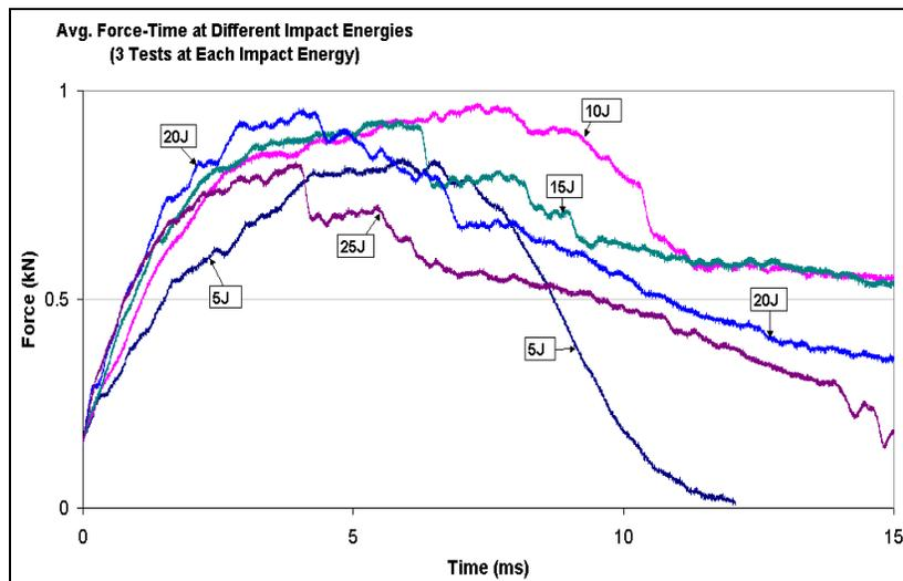
Figure 2. Force vs. Time response for foam core
