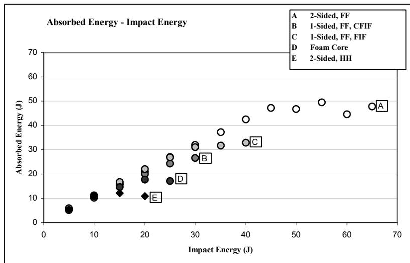
Figure 3. Absorbed vs. Impact Energy for all sample types
