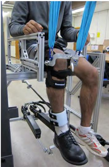
FIGURE 3. ANKLEBOT MOUNTED TO THE CHAIR FOR TESTING THE MECHANICAL IMPEDANCE IN THE MEDIAL/LATERAL ROTATION.
