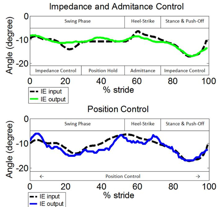
**FIGURE 17:** Input and output (compensated for 75 milliseconds time delay) of the ankle trajectory in IE during a representative gait cycle with admittance and impedance control (top) and position control (bottom).
