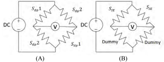
**FIGURE 3:** A: Strain gauge placement in the Wheatstone Bridge for DP torque estimation. Two strain gauges were used for push-off DP torque estimation ( $S_{DP1}$ ) and two strain gauges were used for DP heel-strike torque estimation ( $S_{DP2}$ ). B: Strain gauge placement in the Wheatstone Bridge for IE torque estimation. Two strain gauges are used for push-off IE torque estimation ( $S_{IE}$ ).
