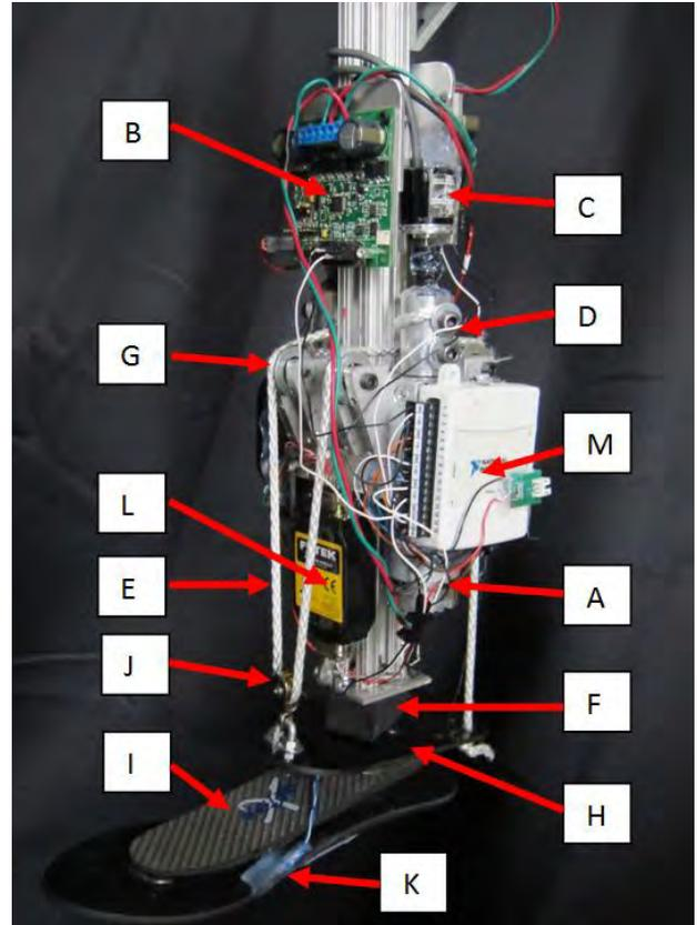
**FIGURE 1:** Two-DOF ankle-foot prosthesis prototype.
