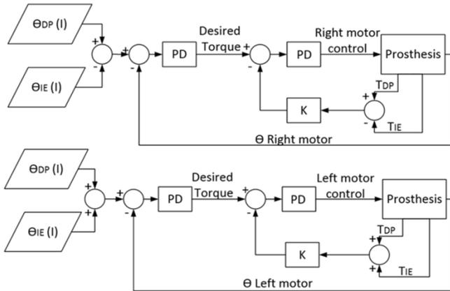
**FIGURE 5:** Impedance controllers for the left and right motors. The reference angle for the left motor controller is the sum of the DP and IE angles, while for the right motor controller is the difference between DP and IE angles. The torque feedback in the left motor controller is the sum of the DP and IE torques, while for the right motor controller is the difference between DP and IE torques.
