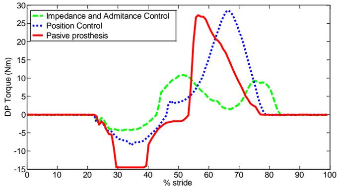
**FIGURE 14:** Ankle external torque in DP during a representative gait cycle with different control strategies. Negative torques induces plantarflexion (heel-strike) and positive torques induces dorsiflexion (push off). With the passive prosthesis, the data acquisition system saturates during heel-strike at -15 Nm torque.
