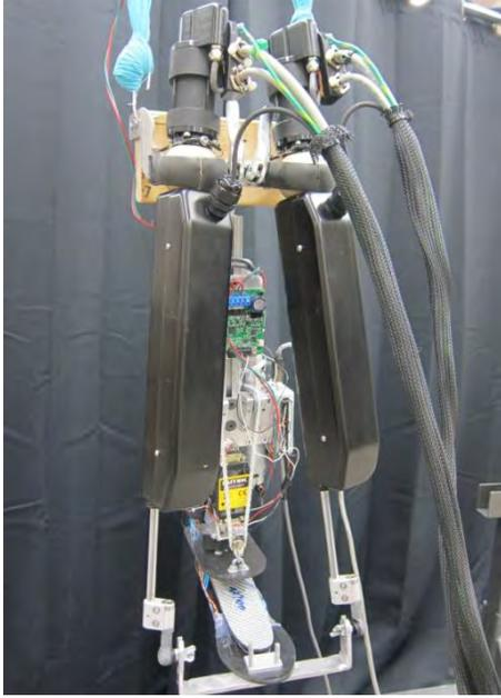
**FIGURE 7:** Ankle-foot prosthesis attached to the Anklebot.
