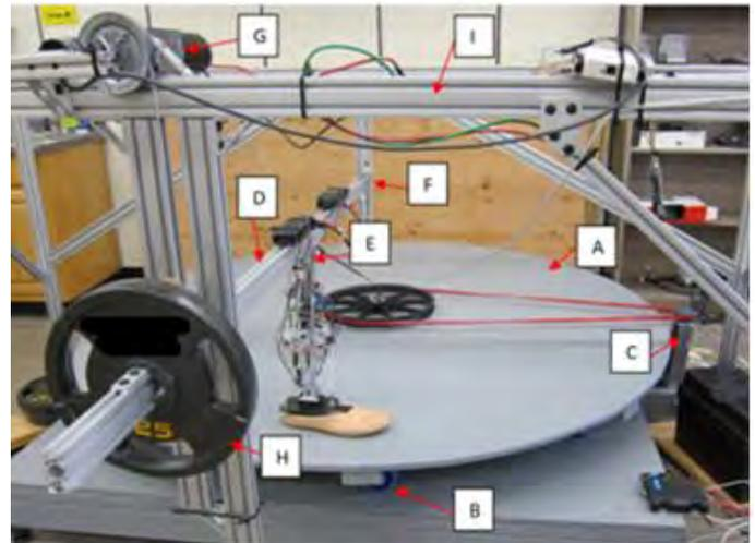
FIGURE 12: Circular treadmill and its main components.
