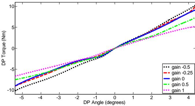
**FIGURE 8:** DP torque-angle relationship in the prosthesis with impedance control and different torque feedback gains. Negative angles are plantarflexion, positive angles are dorsiflexion.
