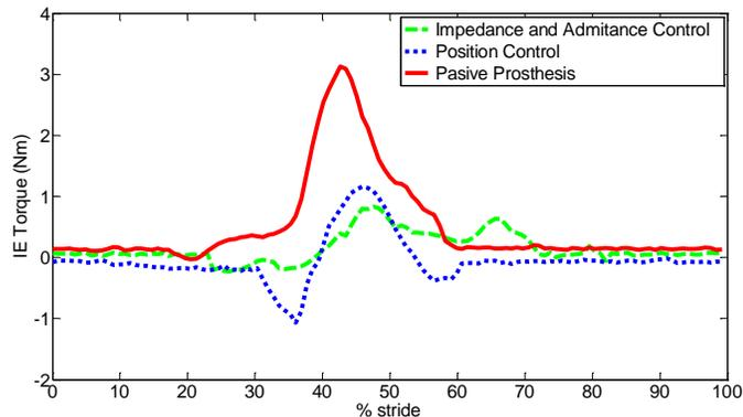
**FIGURE 15:** Ankle external torque in IE during a representative gait cycle with different control strategies. Negative torques induces eversion and positive torques induces inversion.
