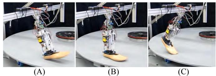
FIGURE 13: Circular treadmill and prosthetic ankle foot robot. A- Heel-strike. B- Flat foot. C- Push off.
