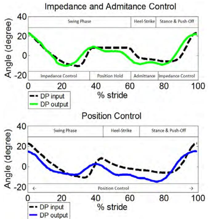
**FIGURE 16:** Input and output (compensated for 75 milliseconds time delay) of the ankle trajectory in DP during a representative gait cycle with admittance and impedance control (top) and position control (bottom).
