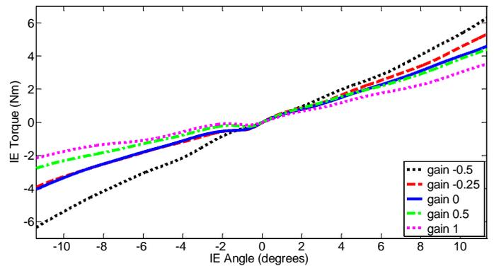
**FIGURE 10:** IE torque-angle relationship in the prosthesis with impedance control and different torque feedback gains. Negative angles are plantarflexion, positive angles are dorsiflexion.
