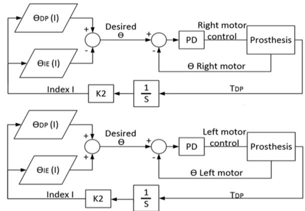
**FIGURE 6:** Admittance controllers for the left and right motors. The reference angle for the left motor controller is the sum of the DP and IE angles, while for the right motor controller is the difference between DP and IE angles. The admittance controller uses the torque feedback in DP to update the lookup table index  $I$ .
