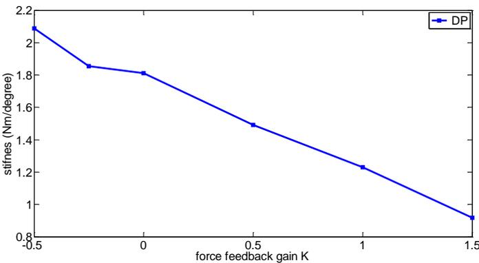
**FIGURE 9:** Ankle stiffness in DP at different DP torque feedback gains.
