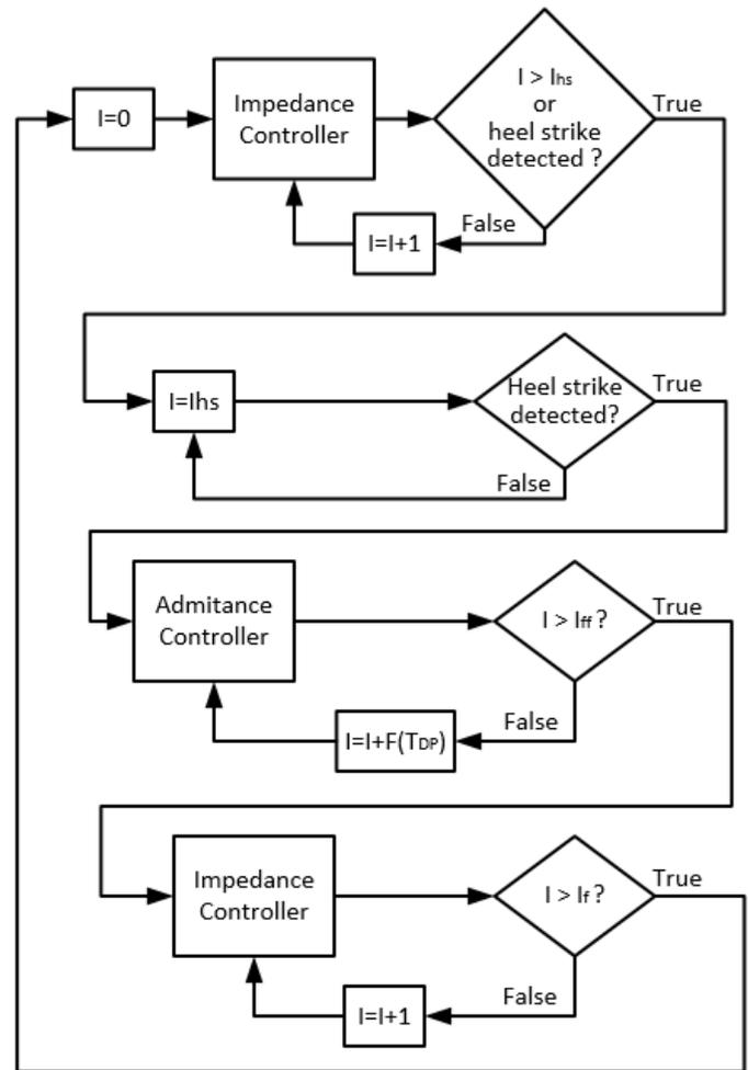
**FIGURE 4:** Finite-state machine to switch between impedance and admittance controllers. In the admittance controller the increment of the index (I) is a function of the external torque disturbance  $T_{dp}$ .
