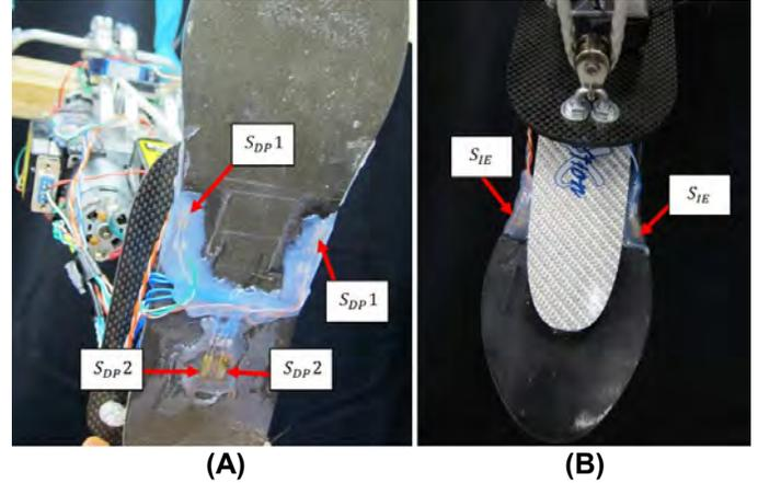
**FIGURE 2:** Strain gauge placement in the prosthesis. A: For DP torque two strain gauges were used for push-off torque estimation ( $S_{DP1}$ ) and two strain gauges were used for heel-strike torque estimation ( $S_{DP2}$ ). B: For IE torque two strain gauges are used for push-off IE torque estimation ( $S_{IE1}$ ).
